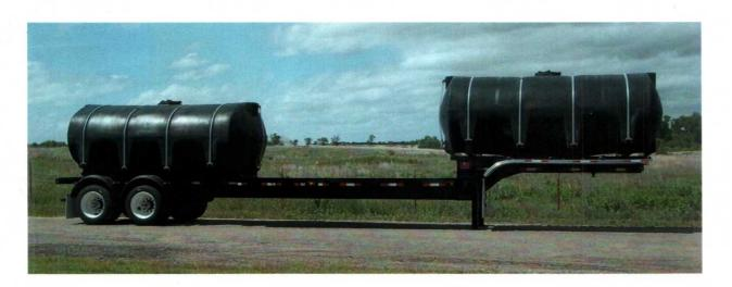
Neville Built offers double tank trailers in standard lengths of 40' or 42' (shorter or longer lengths can be custom built also). The standard 42' has a 15' long by 102" wide working deck space for a pump, mixing equipment, chemicals, seed or whatever else may be needed. Tandem axle configurations in spring or air-ride, as well as spread axle or tri-axle options are available.
