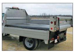
**OPTIONAL** contoured, tapered headsheet is aerodynamically shaped to complement the new cab designs and increase visibility.
