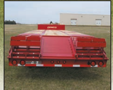
Twin Ramps Standard on Beaver Tail Trailer
