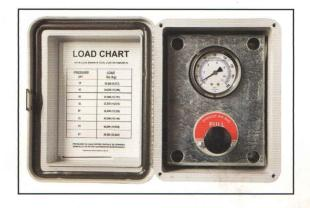
Manual dump valve and pressure gauge with a weather tight box is standard with SAF Holland CBX-23 Fusion air-ride suspension.
