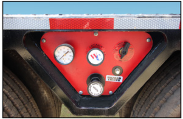
Suspension Controls in Bolster
