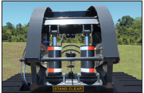
51 ton 8" Bore Lift Cylinder
