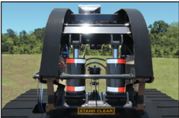
55 ton 9" Bore Lift Cylinder
