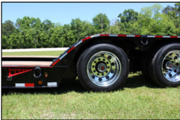
Rounded Bogie Design with Triple Web
