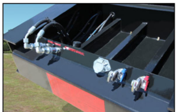
Recessed Electrical and Hydraulic Connections
