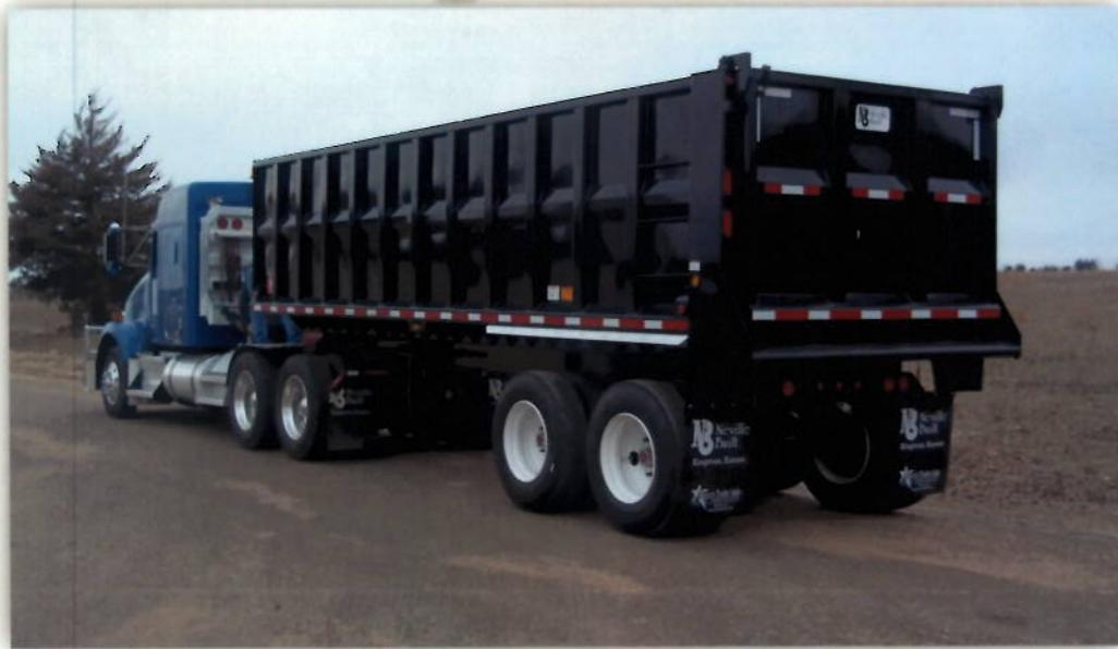
Neville Built full frame steel end dump trailers are available for your hauling needs. We offer a variety of sidewall height options in lengths of 24', 26' and 28'. Standard suspension is spring, however, air-ride or air-ride lift axles are available. We also offer a variety of tarp systems.
